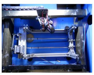
14. Unplug the Y Axis Motor and connect the rotary axis cable (already connected in the picture)
