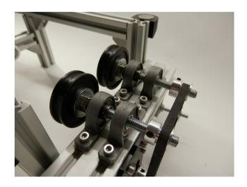
11. Mount the small white wheels on the other side. Use the spacers and make sure you use the M5 T block not the standard M4 blocks
