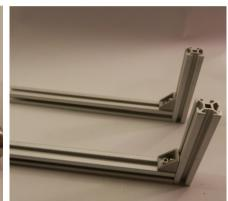
2. Connect the ends of the two 25cm pieces with a 17cm 2020 profile. Don't forget to insert some T-Nut blocks on both sides beforehand like in the picture.
