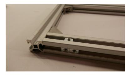
3. Mount the motor and two corner brackets to the 2040 aluminium. Use some sandpaper or a file to trim down the small taps on the corner brackets
