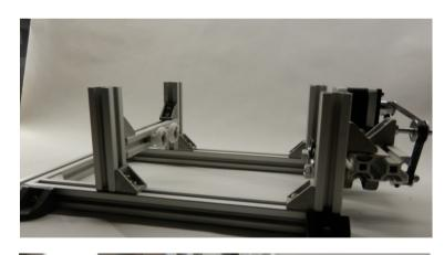
6. Mount the 4 magnet feet with the 4 T Nuts we inserted before.
