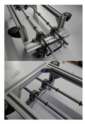
9. Insert the belt and tighten everting up. Make sure everything is square and perpendicular.
