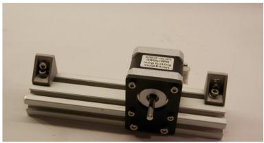
4. Assemble the belt tensioner and mount it to the 2040 like in the next picture(don't forget to remove the small tap on the corner bracket)
