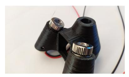
3. Insert the screw (the screws holding the lasers can be installed later after testing if the beams hit the right spot, screws might not be necessary)
