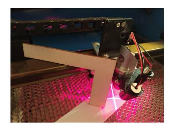
10. Now you can check if the lasers are aligned with your co2 beam. Take a piece of paper and shoot a short test beam. Now you can adjust the laser lines by hand and secure them with the screws.
