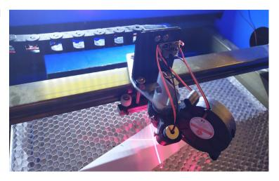
8. Wiring: The Laser run on 5V. The Fan runs on 24V. You can get both voltages from the power supply.
