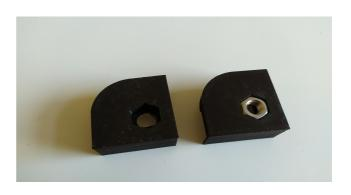
8. Screw the corner pieces into the treaded rods.
