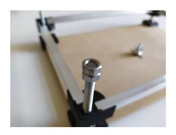
11. Run the belt around the table an tighten it with the belt tensioner (putting the table on the side and having a second person makes it easier)
